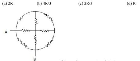
14. Eight resistances each of 5 ohms are connected as shown. Equivalent resistance between A and B is
